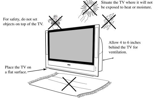
Do not place the TV on a surface that will block the air filters located underneath the set.
